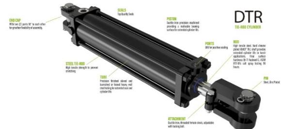
Typically these cylinders have end caps that are attached to the end of the cylinder barrel via a rod that is inserted through holes in the end caps. Once through the hole, the rods are secured in place by nuts threaded onto the end of the rod.
