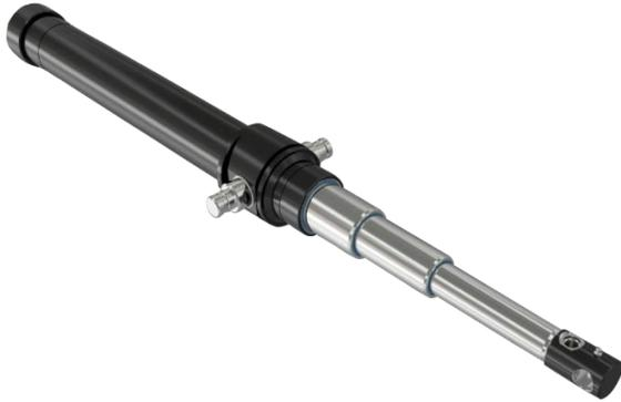
**Telescoping Cylinders** are comprised of multiple tubular sections that fit together. The tube-based sections function independently as small cylinders. By adopting this design, it is possible to vary the size of the individual tubing sections to create long overall cylinders. At the same time, the ability to telescope down into a small footprint makes this type of cylinder desirable for mobile applications in which the cylinder mounting area is restricted.
